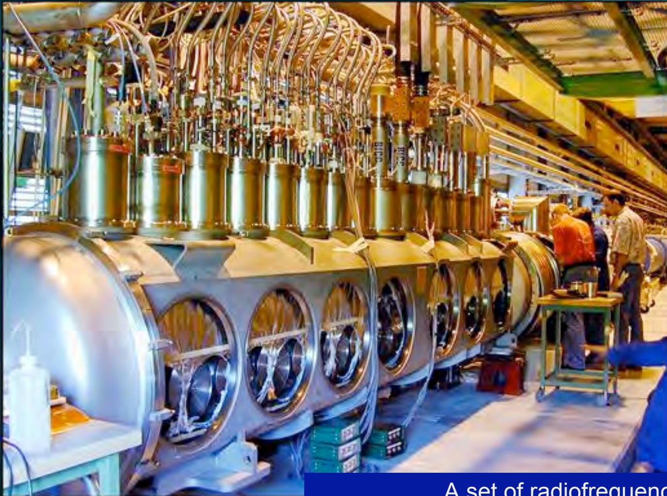
A set of radiofrequency cavities
